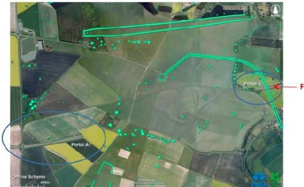
Fig. 3 shows a map of the 1.9 km option from the Snasha/1 & Young report, fig. 7, p. 34. "A.303 2.9 km bored tunnel (Tcta 2014, Appendix D, 2or'. Highlighted in blue by the authors are the two portals A1 and E. If the Eastern portal (currently proposed point 'F') was further to the east of the King's farrow ridges (point 'F') it would not cut through the Avenue and this would significantly reduce the adverse impacts on the Avenue which is a major feature of the World Heritage site.
